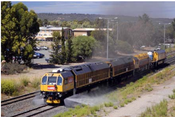
Photo – RG9 Rail Grinder at Mile End
