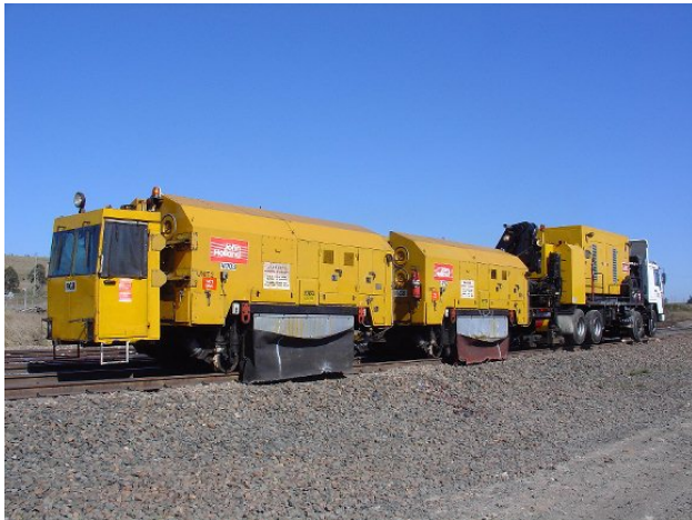
Photo – RG8 Rail Grinder
