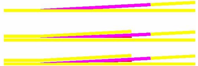
Figure 13 – Diagram of Normal Switch (top) and the Geometric Problem to be Overcome in Achieving Internal Checking
