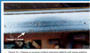
Figure 25 - Flaking of railway surface checking defects with minor spalling
