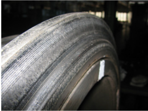
The German solution for dual running – a mixed profile tramtrain wheel – standard rail wheel back-to-back, with a wider section for tramway running towards the tip of the flange (Karlsruhe).
