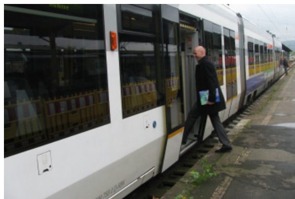
Standards for platform gaps and step heights appear to be less rigorous than in Australia (Alstom Cidatis tramtrain, Kassel)
