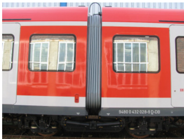
Articulated railcar sets reduce overall train weight and length ...
