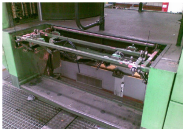
Complex step mechanisms accommodate platforms of differing heights – top deck removed for photo, a movable step extends and lowers for low platforms (Hanover tram network)
