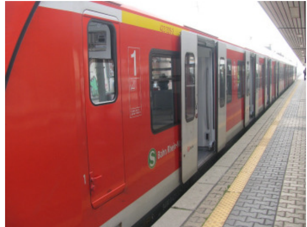
Rolling stock typically has straight sides. Plug doors optimise the provision of windows (S-bahn, Frankfurt)
