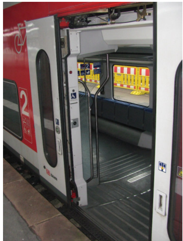
On double deck cars, the entry and lower saloon are typically at platform level (regional service, Kassel)
