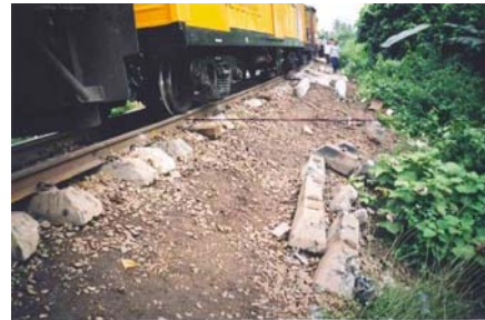
Derailed of coal train KA BBR 21 at South Sumatra 17 December 2003 7 coal train derailed (28 axles)
