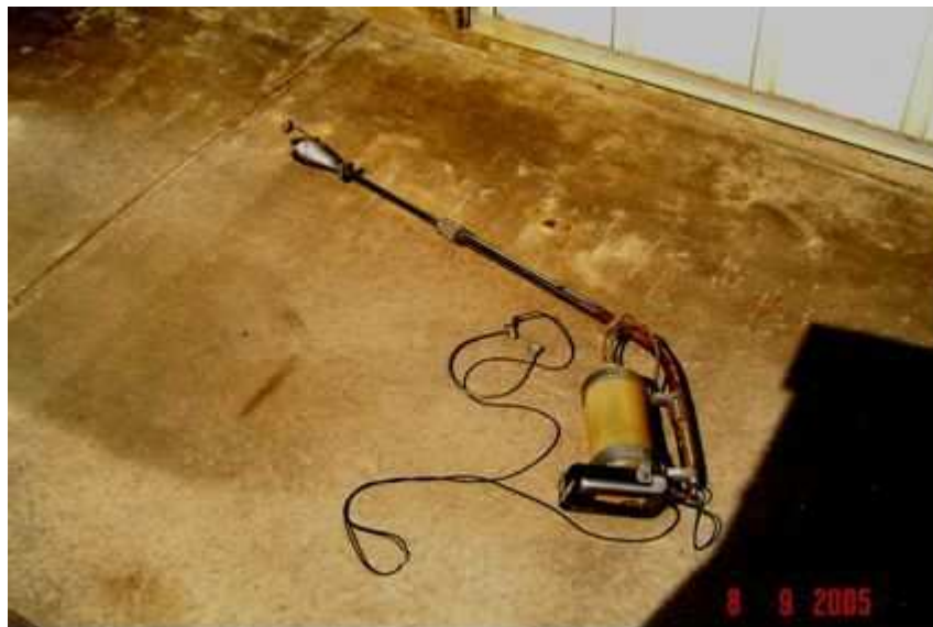
“Flawtone” Ultrasonic Hand Tester.
