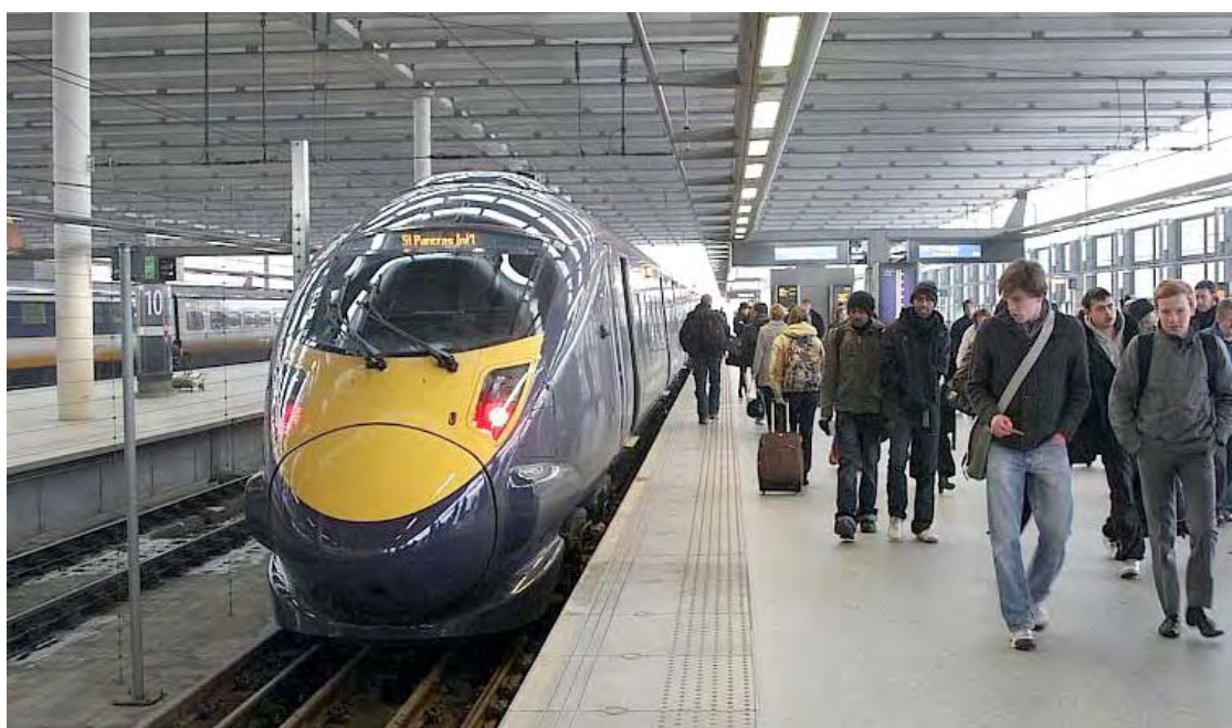
In the south east of England, mid-range high speed (225km/h) commuter and regional services share tracks with international HSR Eurostar services on the high speed corridor between St Pancras and Ashford.
