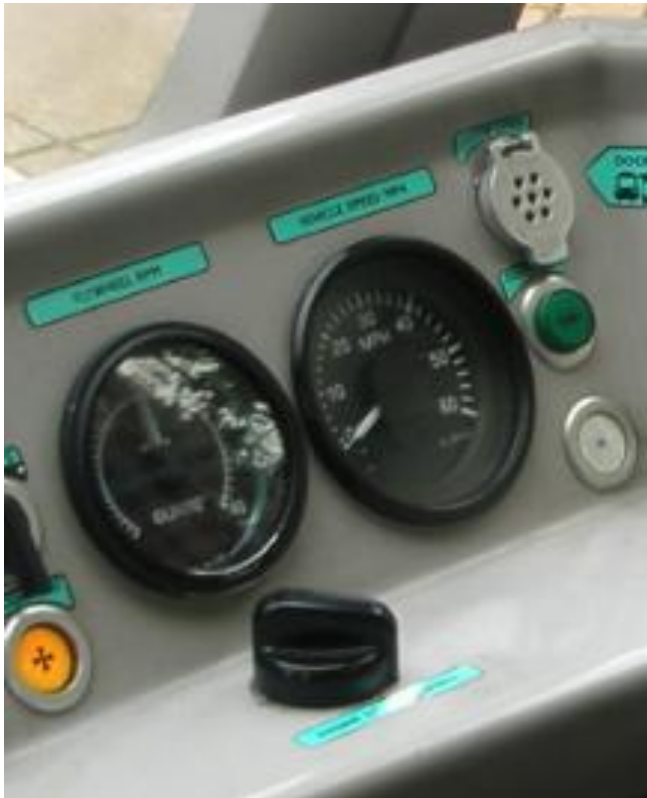
An unusual feature in a train – a flywheel speed indication
